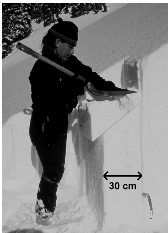
Figure 1: The compression test is a stability test. The column of snow is loaded by repeatedly tapping on the shovel. The first ten taps are with the fingertips, moving the hand from the wrist, followed by ten taps moving the forearm from the elbow and finally ten taps moving the whole arm from the shoulder.
