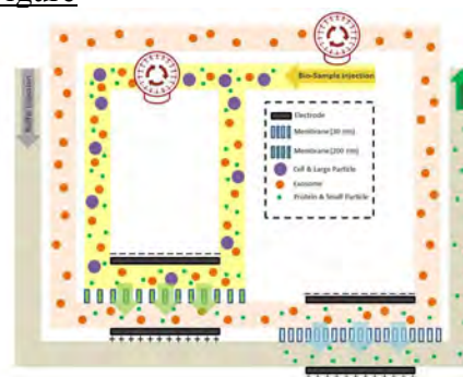
Fig.1. Schematic of the proposed microfluidic method for exosome isolation
