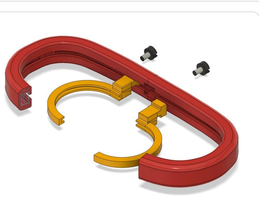
Figure 1. Trial Lens Frame CAD Model
