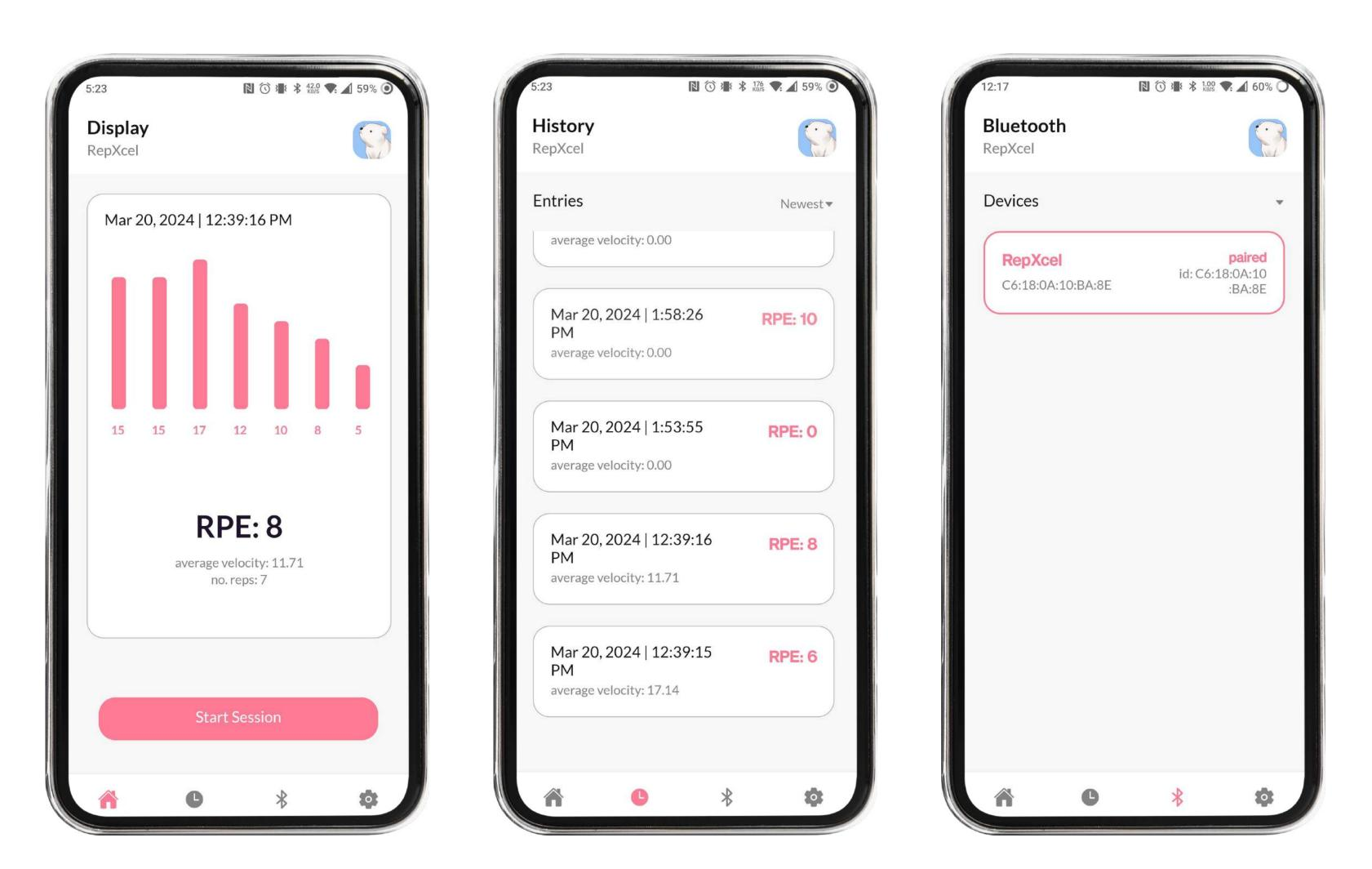
The app is created using React Native with TypeScript. The back-end is hosted on AWS Amplify. The app offers many features such as: user authentication, Bluetooth connectivity, RPE calculation, and data visualization and synchronization.
