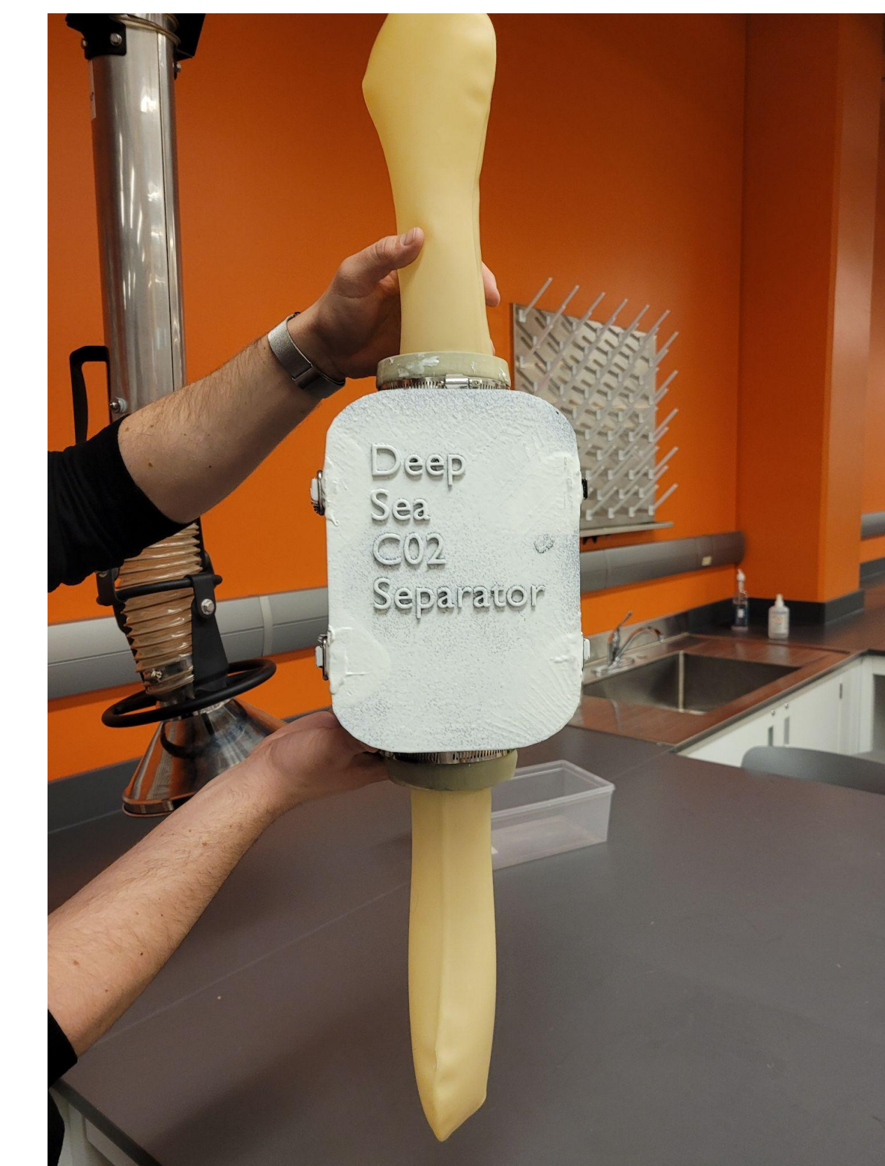
Fig 5. The design of the outside of the prototype. The latex balloons are pumped up using the air valve located on the inside of the device.
