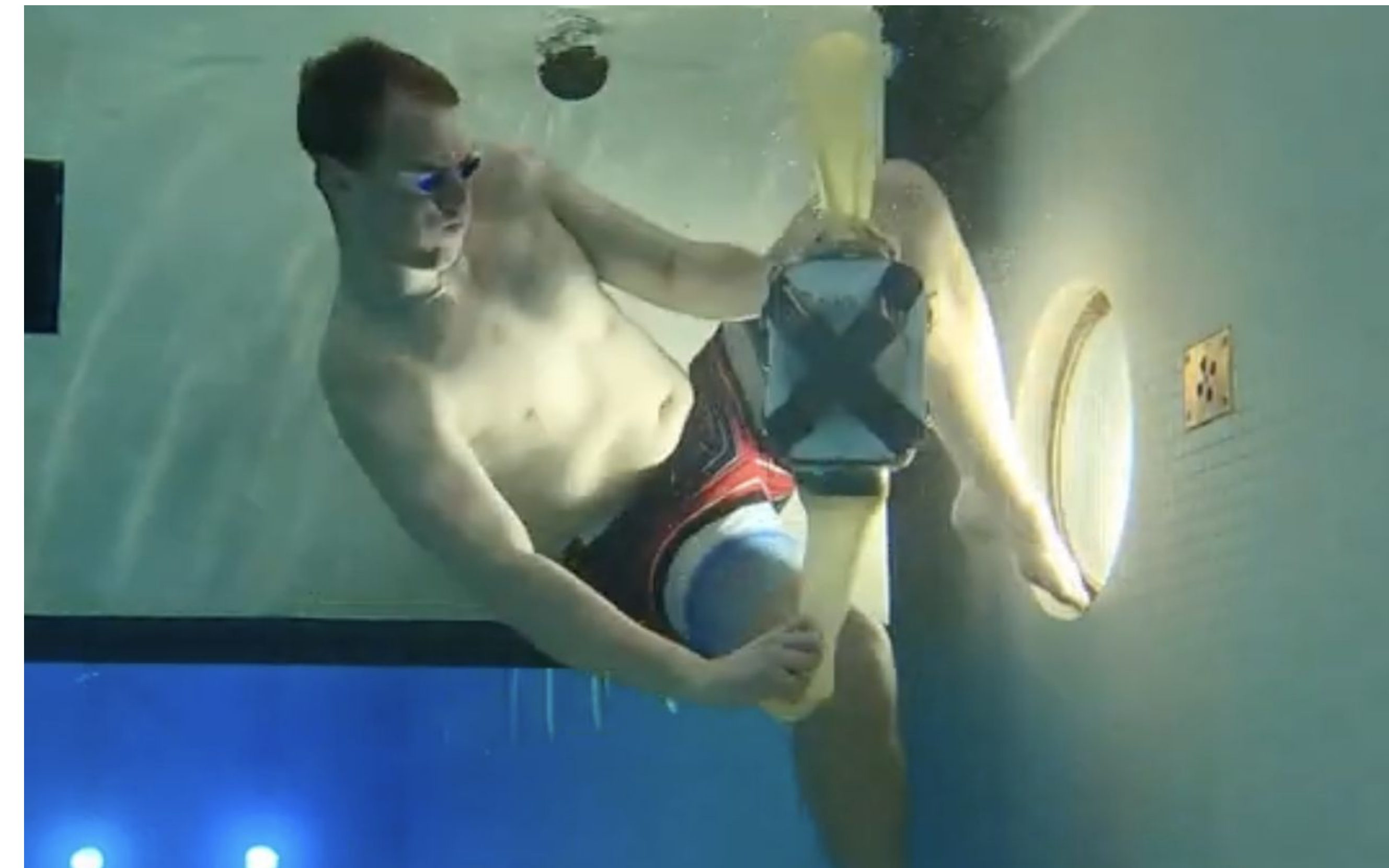
Fig 3. The final test for the prototype in a U of C pool. The depth sensor was able to trigger the valve to close at the depth we specified, 1.5 m. The trigger depth can be adjusted for a larger scale test. A weight was also taped on to help sink the device.
