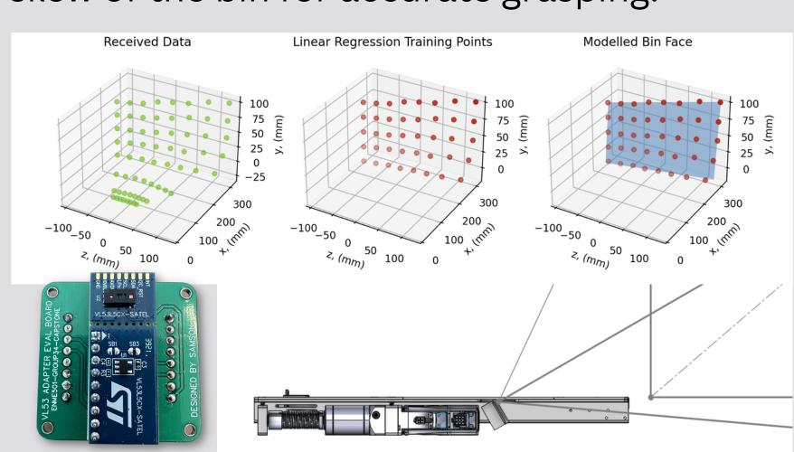
Using the VL53L5CX multi-zone lidar sensor, with our custom firmware, we detect the bin within ~2.5mm accuracy and ~2.5 degree accuracy.
